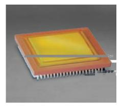
The Moog Broad Reach BRE440 CPU meets the requirements of a wide variety space and high reliability applications. The BRE440 CPU is a fully radiation hardened implementation of the PowerPC 440 processor core in a true System-On-a-Chip design, including floating point unit.
