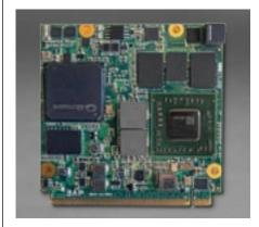
The e2000/e2100 heterogeneous computing product families are radiation tolerant high-performance compute modules for onboard data processing. The products have spaceflightheritage and uses low power embedded x86 compatible AMD® G-series SOC products from the 1st, 2nd, and LX families. The SOC is paired with a powerful Microsemi® SmartFusion2™ FPGA which provides IO expansion and board supervisory management through IP core state-machines or embedded ARM® Cortex™ M3 micro-controller.
